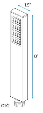
Flow Rate: 2.0 GPM / 7.6 LPM
